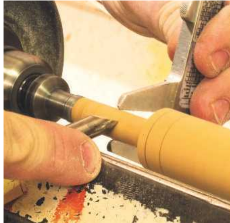
▲ Pic.29 Make sure that the spigot is long enough to go all the way through the head. Using Vernier callipers for accuracy, turn it down to the exact size to fit through the hole
